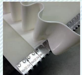
Rivet fastener with a Compart™
